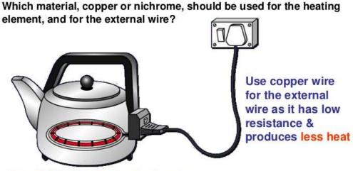
Use nichrome wire for the heating element as it has high resistance& produces a lot of heat
